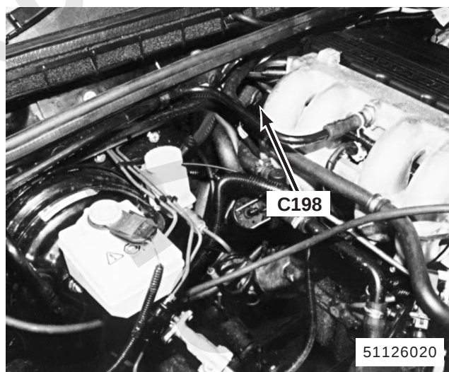
68. RH rear corner of engine compartment (MFI-T16)
