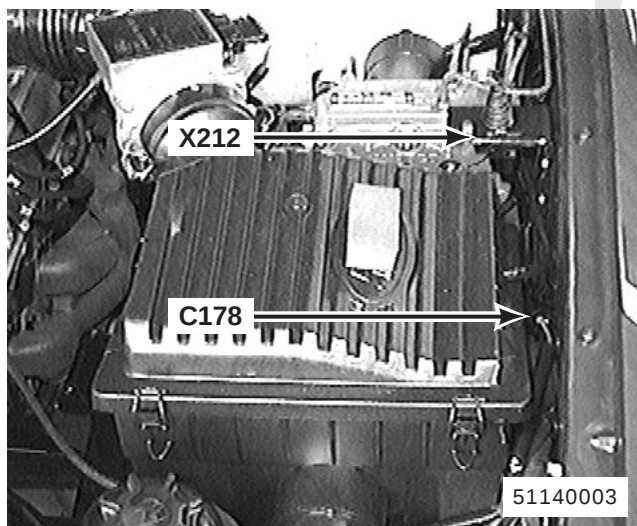
227. LH side of engine compartment X212 Alarm Bonnet Switch C178 (2-B)
