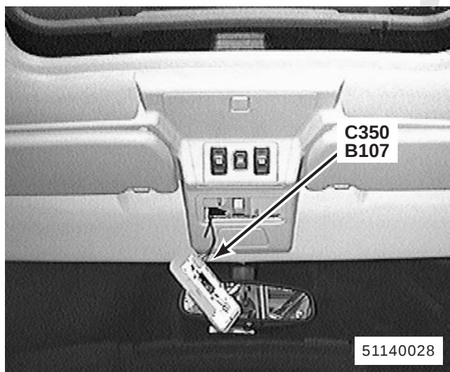
131. front centre of roof B107 Front Interior Roof Lamp C350 (3-W)
